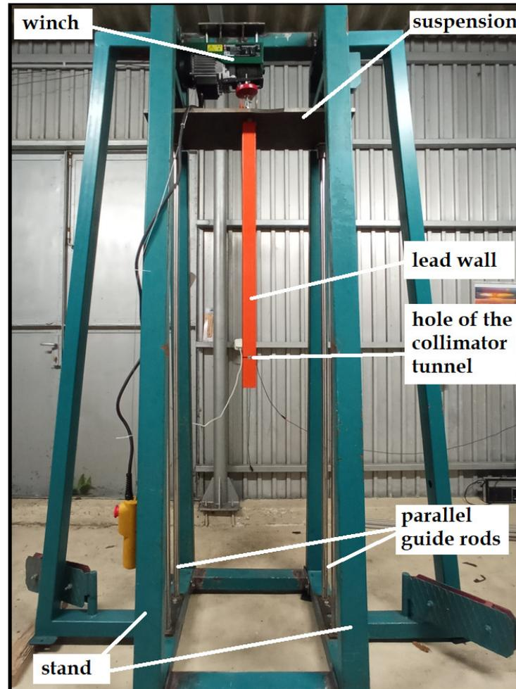
*Figure 3: A side view of the gamma-guillotine, showing the design of the stand, the suspension, the controlled movement of the lead wall with parallel guide rods and winch, as well as the hole of the collimator tunnel*
