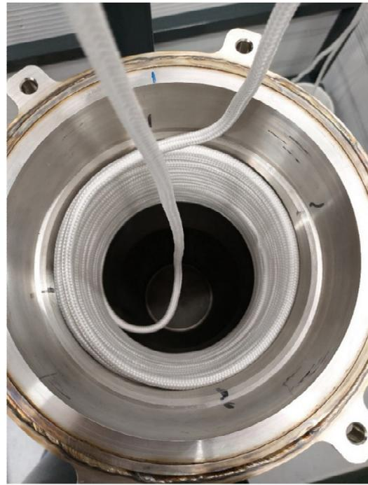
Figure 4: Test induction coil placed in the DN 200 pipe
