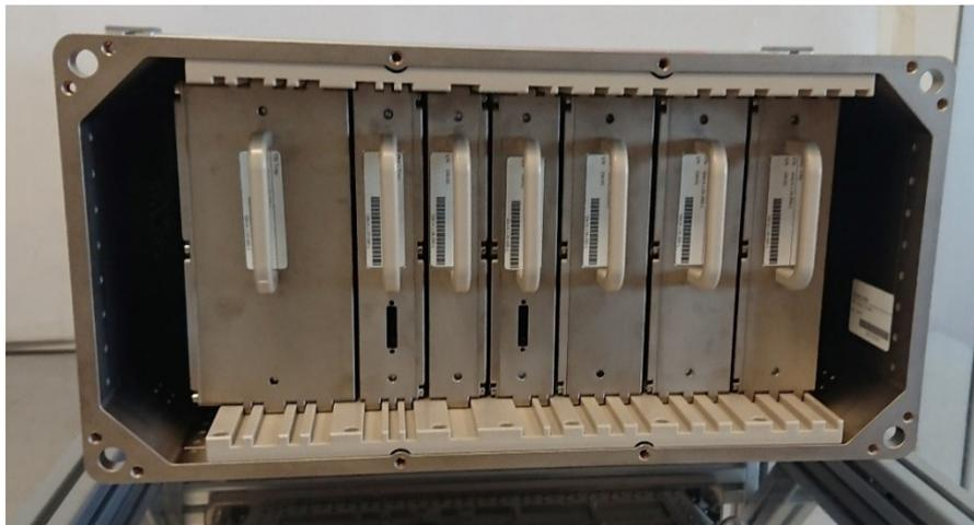
Figure 1: IDA Payload internal structure after front panel opening. The trays from left to right are: TRITEL, Avionics modules (Payload Power Converter Module, Payload Digital Processing Module, Payload Memory Module), PDS, MediPix, and EAD
