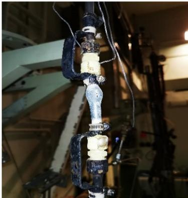
Figure 1: Sensor fixing on the tube
