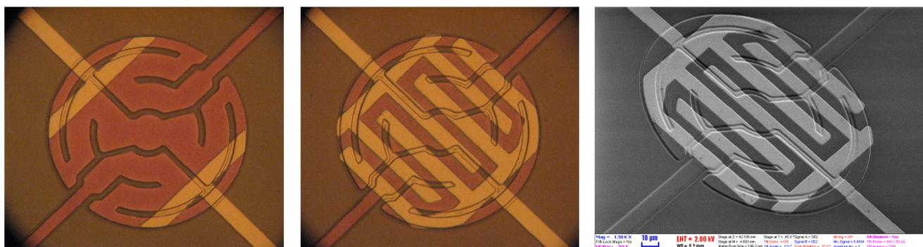
Figure 1: Microheaters with different electrodes for performance testing the sensitive materials
