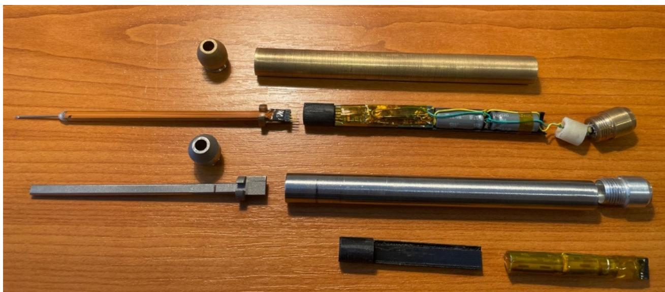
*Figure 1: "Smart scalpel" surgical force measurement tool: head and electronics with covering*
